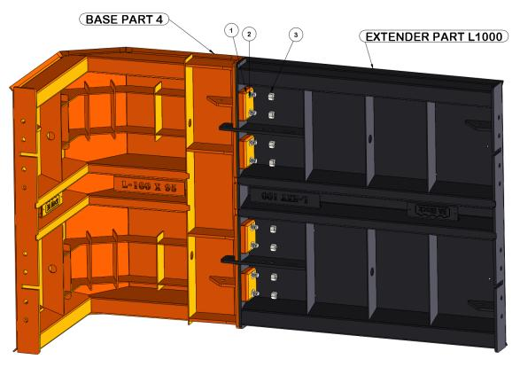
Align the BASE PART 2 to EXTENDER PART L1000 and put bolts (pos.1), CONNECTION PART 1, washers. Screw the nuts by hand to the end.
