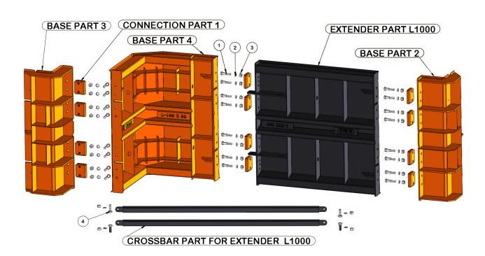
Align the BASE PART 4 and EXTENDER PART L1000 and put bolts (pos.1), CONNECTION PART 1, washers. Screw the nuts by hand to the end.
