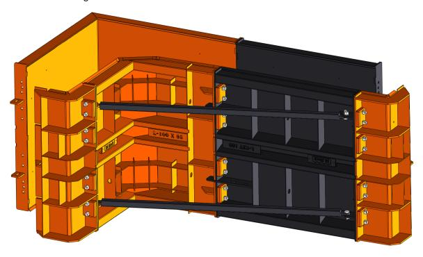
Align the two half of mold and put the CONIC PIN to guide them to final position.
