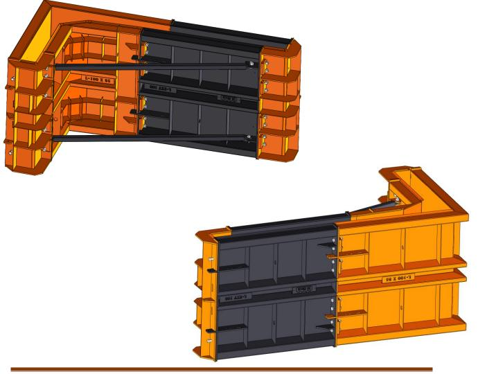
Put the 4 wedges in position and with hammer hit the wedges and conic pins to completely close the mold.
