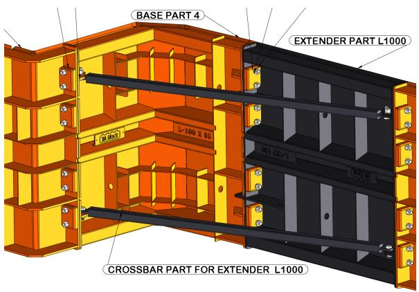
STEP 3: Assembling the two half of the mold.
